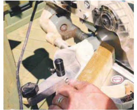
STEP 4. Setting the miter saw to 30°, cut a mitre and then rotate the leg
